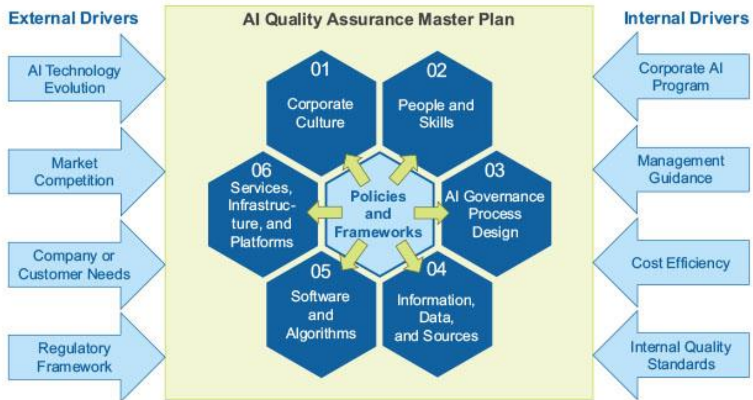
Figure 1: Focus areas in an AI quality assurance master plan, including internal and external drivers.
